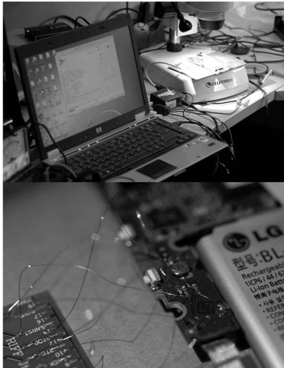
FIGURE 4.38 Joint Test Action Group extraction using Octoplus
