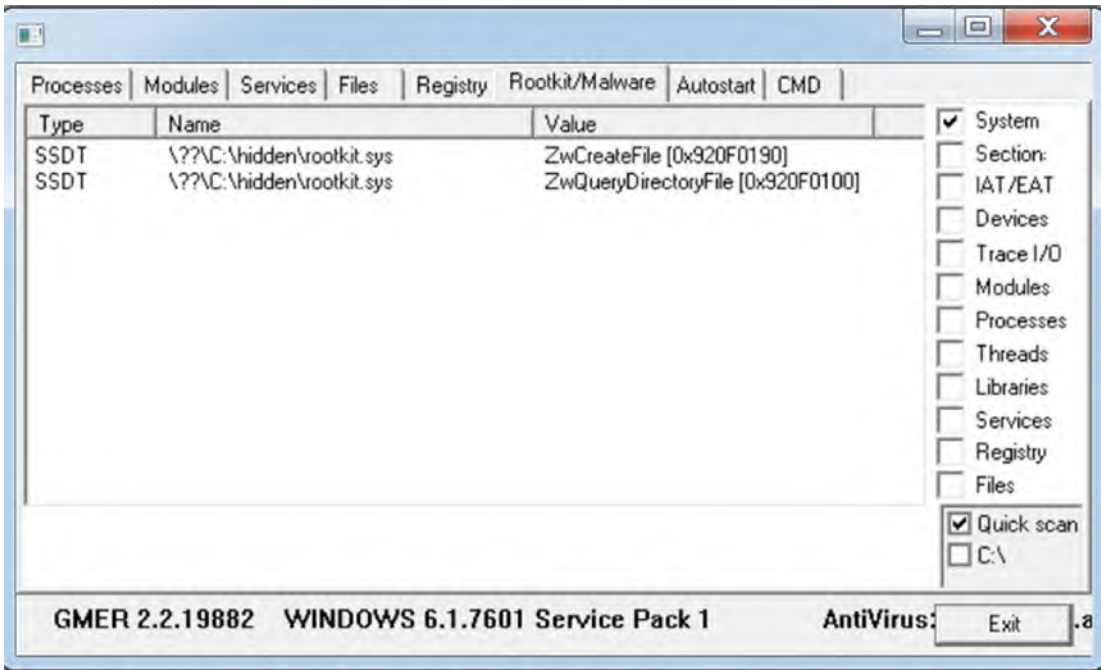
Figure 11-27. GMER identifies that we have an SSDT rootkit installed on the system
