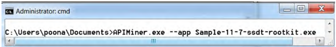
Figure 11-25. APIMiner running the SSDT rootkit from our exercise Sample-11-7-ssdt-rootkit
